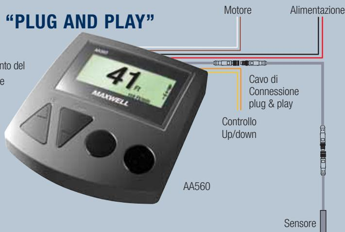
**TUTTI I SALPANCORE MAXWELL SONO PREIMPOSTATI PER IL CONTACATENA, CON MAGNETE INSTALLATO E FORO PER IL SENSORE**
